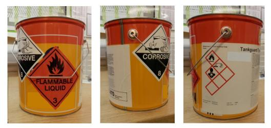
**Problem:** This packaging contains a product classified as UN 3470 PAINT, CORROSIVE, FLAMMABLE. Two transport labels, Class 8 and Class 3, are therefore required to be displayed on the packaging. (The product is also classified for supply as a respiratory and skin sensitizer under GHS.)
