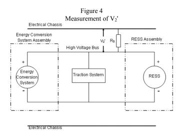
Note 1: The standard known resistance  $R_o$  (in  $\Omega$ ) should be the value of the minimum required isolation resistance ( $\Omega$ /V) multiplied by the working voltage (V) of the vehicle plus/minus 20 per cent.  $R_o$  is not required to be precisely this value since the equations are valid for any  $R_o$ ; however, a  $R_o$  value in this range should provide a good resolution for the voltage measurements.
