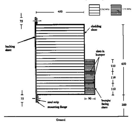
Barrier width = 1 000 mm. All dimensions in mm.
