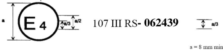
The above ..... pursuant to Regulation No. 107 under approval number **062439**. The approval number indicates ..... as amended by the **06** series of amendments."
