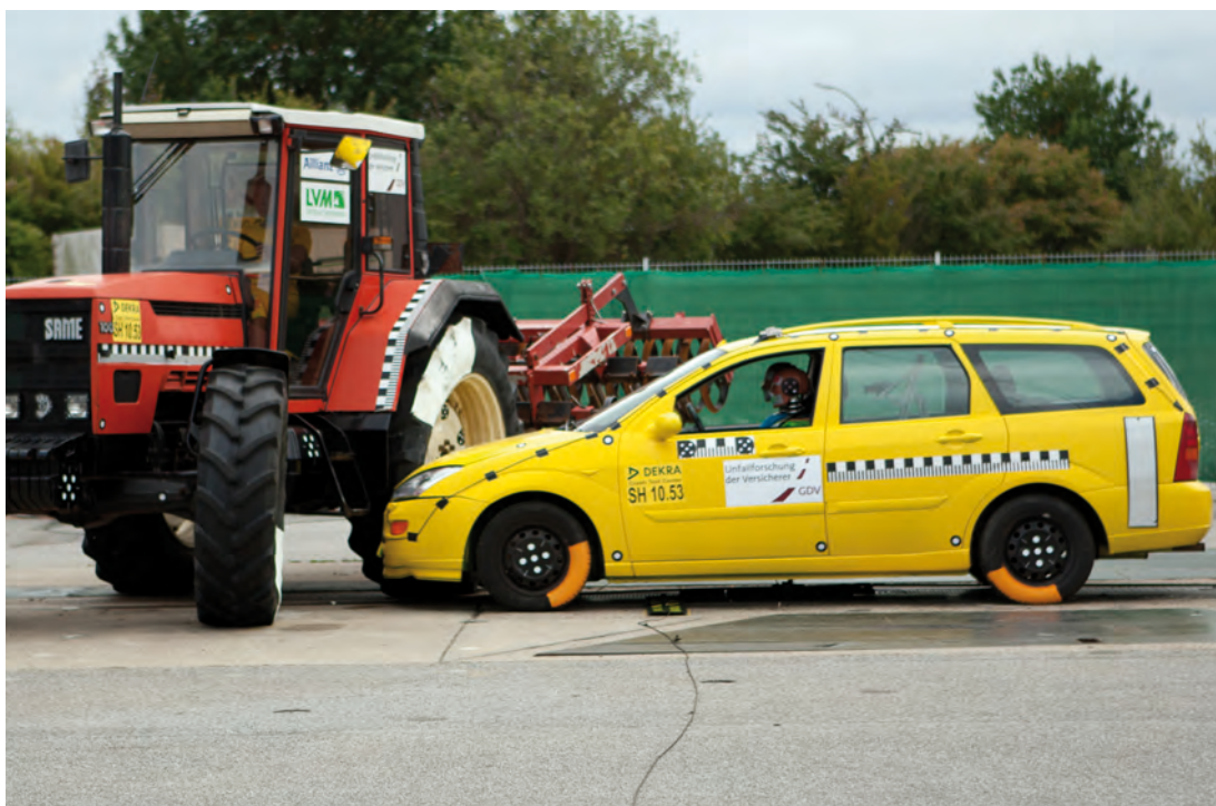
Picture 12: Crash test with tractor vs. passenger car (before the impact)
