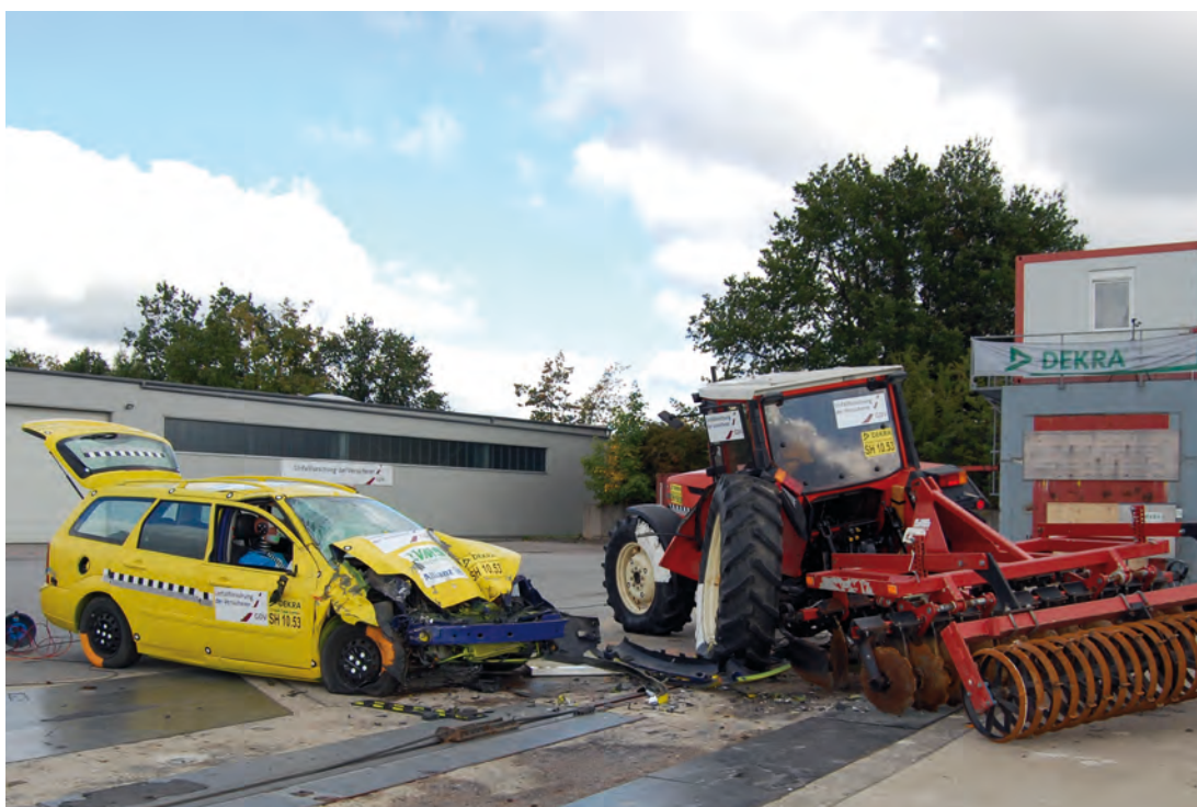
Picture 13: Crash test with tractor vs. passenger car (after the impact)
