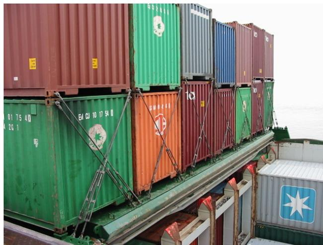
Figure: 2.2 Cell guides and lashing rods on a container vessel
