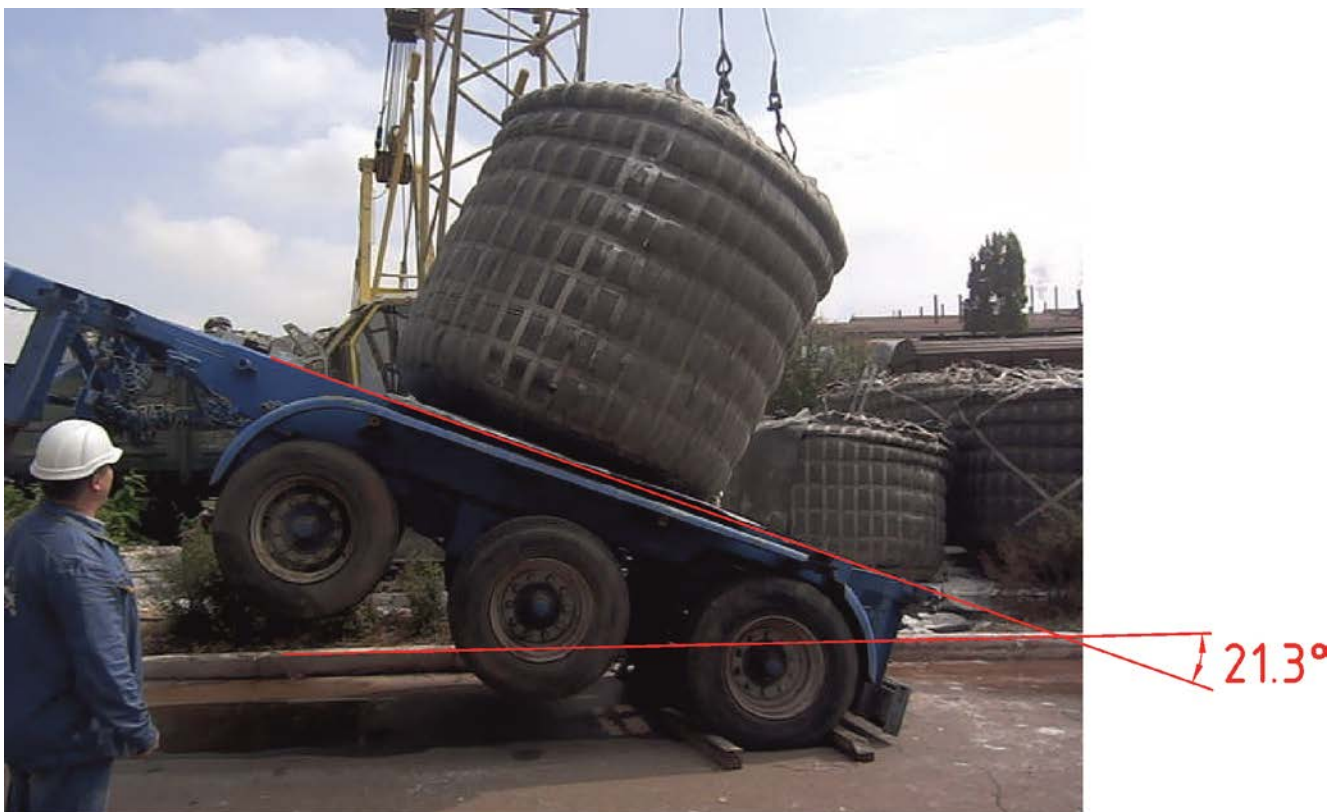
The third container. Video file 3389. Snapshot 1:42/1:50. The platform is tilted up to the angle 21.3 degrees.
