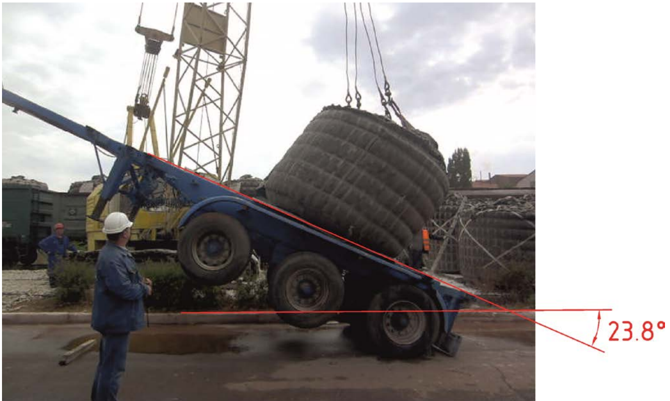
The first container. Video file 3373. Snapshot 3:12/3:22. Platform is tilted up to the angle 23.8 degrees.
