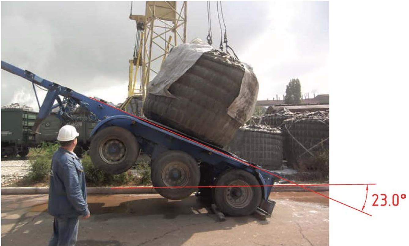
The second container. Video file 3381. Snapshot 2:14/2:20. Platform is tilted up to the angle 23.0 degrees
