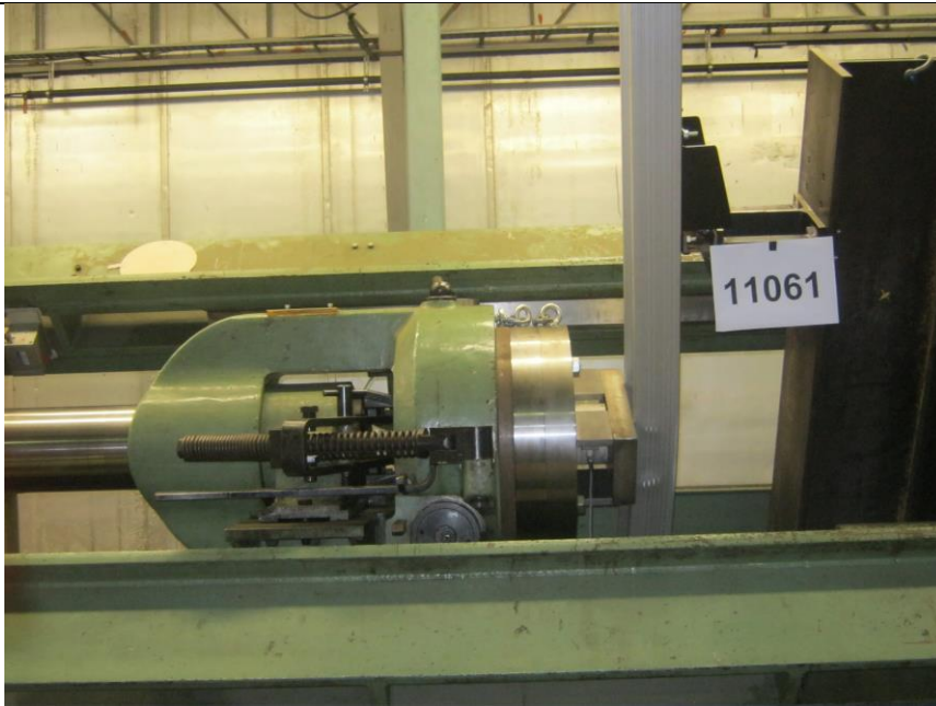
Figure 4: Tension-compression testing machine with aluminium underrun protection and end support
