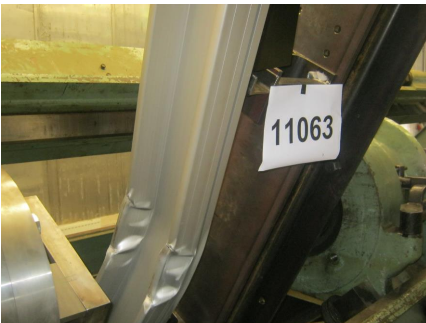
Figure 9: Aluminium section after application of quasi-static load
