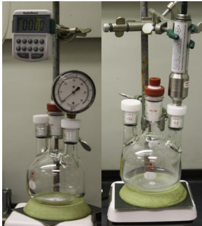
Figure 2 – Reaction apparatus, configured for manual data acquisition (left) and electronic data acquisition (right). In both cases the center port is fitted with a septum to allow fluid injection.
