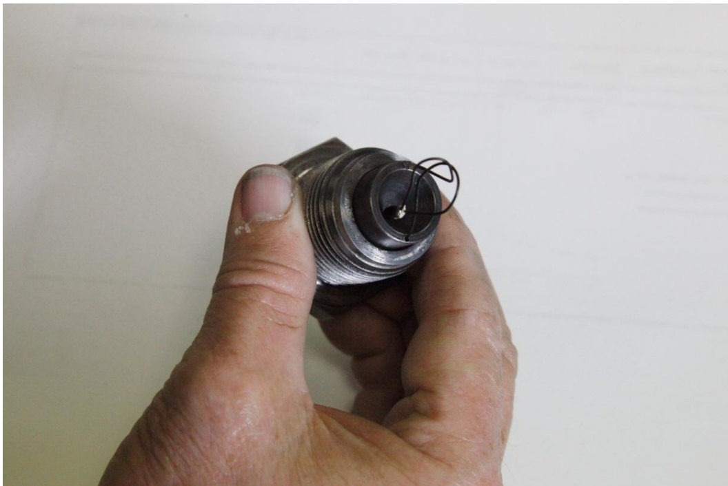
Figure 13: Assembled Modified Firing Plug with Folded Electric Match
