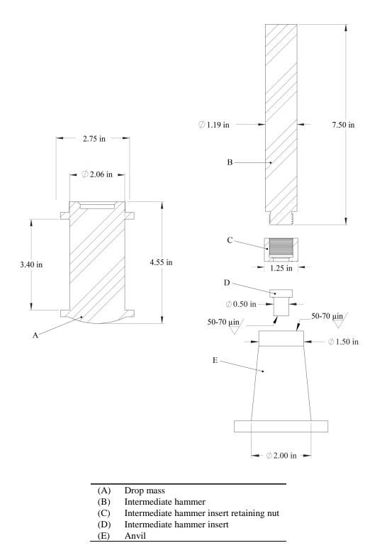
Figure 13.4.7.2: MBOM Impact machine drop mass and target area detail"
