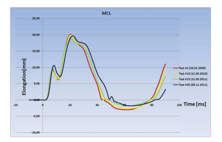
High repeatability during the impact phase Test #20 with slightly different time history curve
