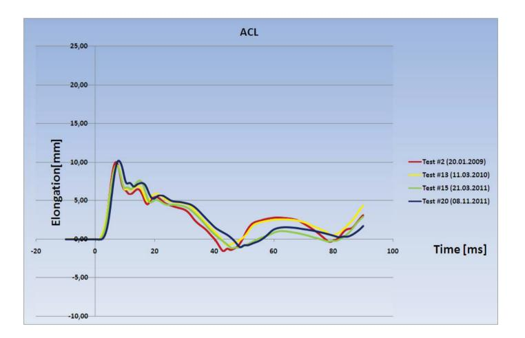
High repeatability during the impact phase Test #20 with slightly different time history curve after the first peak
