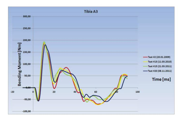
High repeatability during the impact phase (primary impact) Test #2 with highest decay after first peak
