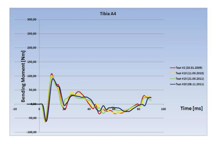
High repeatability during the impact phase (primary impact) Test #20 contributes to a higher scatter and thus a CV of 5,77 % Test #2 with highest decay after first peak
