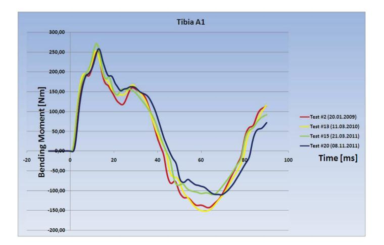
High repeatability during the impact phase Test #2 with highest decay after first peak
