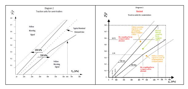
Currently the driver warning signal is not generated until the coupling force control function adjusts the braking performance of the towing vehicle by +/- 150kPa from the "nominal demand line" which is the design braking performance of the towing vehicle relative to coupling head pressure. The proposal from Denmark is to significantly reduce the amount of compensation that may be applied before a driver warning signal is generated.
