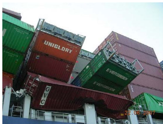
Figure 2.7: The collapse of a container stack may have various causes. One cause could be the overstressing of lashing devices (© KIMO International)
