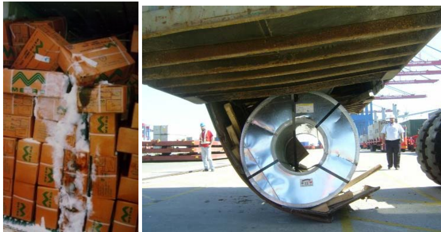
Figure 2.5: Frozen water from leak in roof (left), local overloading of bottom (right)
