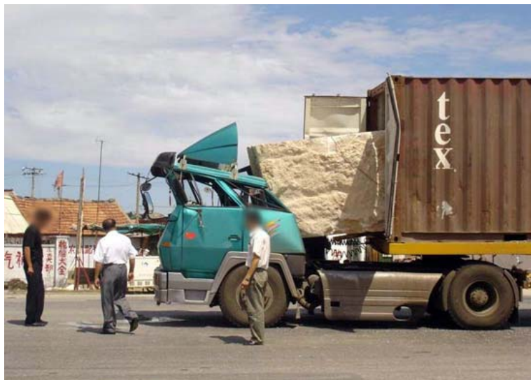
Figure 2.1: Hard braking with lack of longitudinal securing
