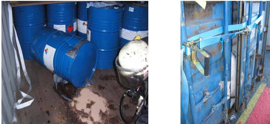
Figure 2.3: Liquid spillage, absorbents applied (left), solid spillage (right)
