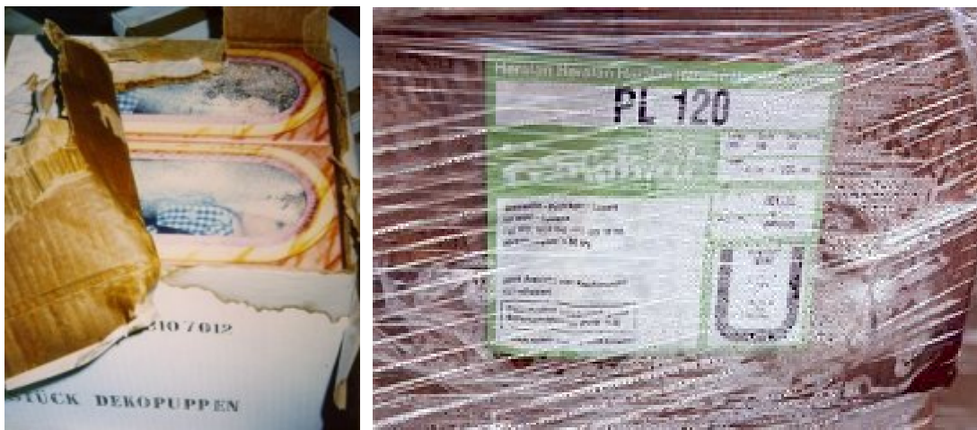
Figure 2.4: Mould damage (left), condensation within plastic sheathing (right)
