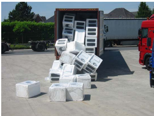
Figure 2.2: Lack of securing at door end (left), on railway wagon (right)
