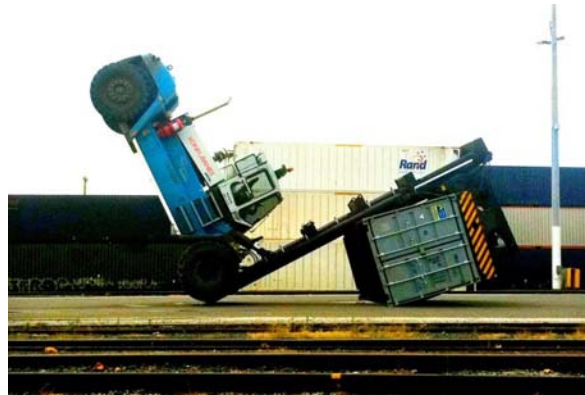
Figure 2.6: A reachstacker is tipped forward by an overloaded container (© abc.net.au)
