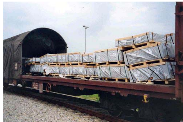
Figure 2.2: Lack of securing at door end (left), on railway wagon (right)
