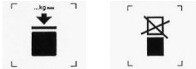
IBC capable of being stacked (stack load indicated in kg) IBC not capable of being stacked
