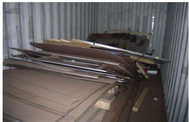
3.2 One of the casual factors found was that the 20ft container load was likely to have been offset to the left. The picture also shows that the strapping securing the cargo within the container has broken despite the container not falling from the wagon. The accident
