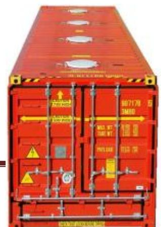
having filling and discharge apertures and fittings and complying with ISO 1496 part 4<sup>14</sup>.”
