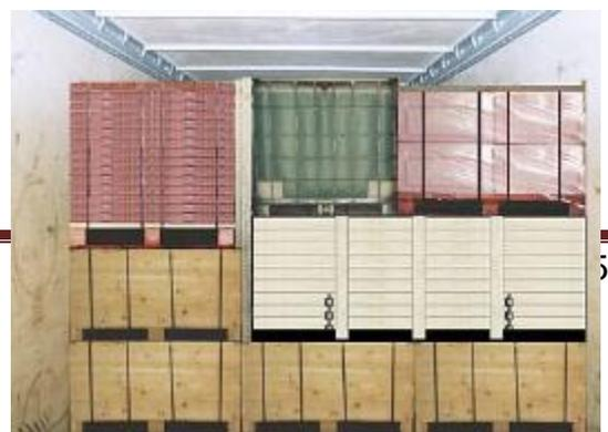
without any time delay. The dimensions, strength and loading capacity of the aids used, such as squared lumber, wooden dunnage boards etc. must ensure that the goods do not suffer any damage during shipping. If necessary, stowage surfaces must be prepared with walking boards, boards, cargo items with a high loading capacity or other usable aids, so that work can be carried out safely and the batches that have already been loaded can be overstacked with other loads.
