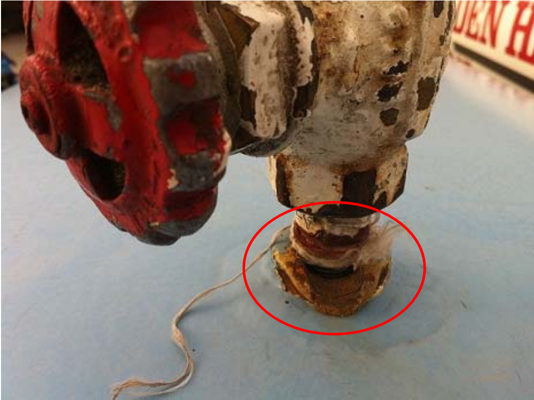
Damaged tank (after a valve was placed to contain the gas leak)
