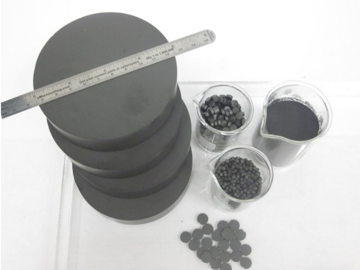
Figure 4 Typical Adsorbent Form Factors
