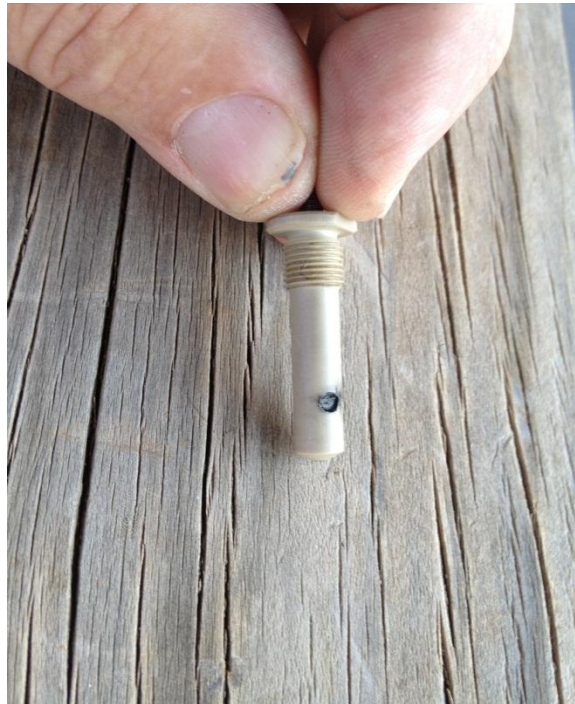
Figure 4. HSL Fixture Plastic Insulated Component Damage
