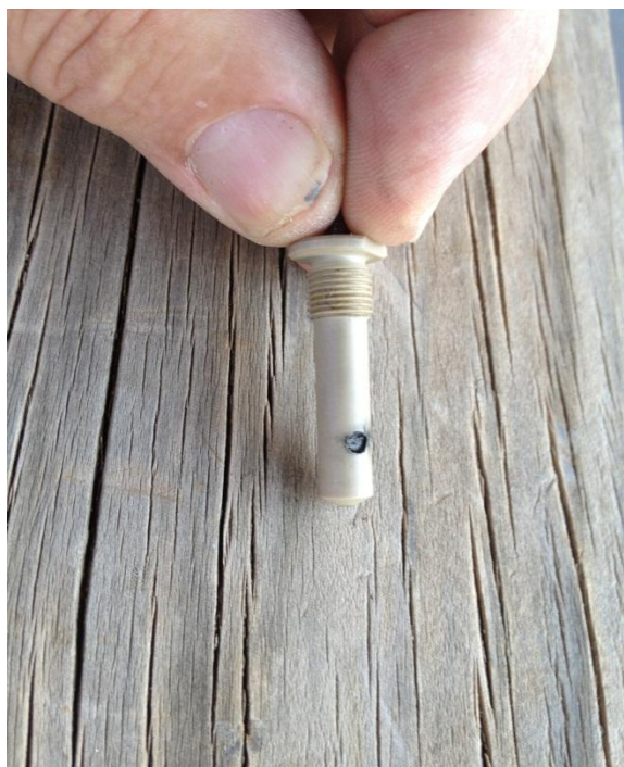
Figure 4. HSL Fixture Plastic Insulated Component Damage
