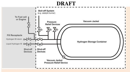
Figure 4. Typical Liquefied Hydrogen Storage System
