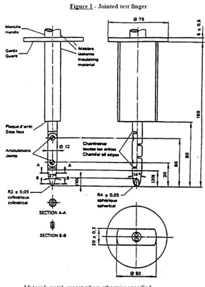
Material: metal. except where otherwise specified Linear dimensions in millimeters Tolerances on dimensions without specific tolerance: on angles, 0/-10' on linear dimensions: up to 25 mm: 0/-0.05 over 25 mm: +/- 0.2 Both joints shall permit movement in the same plane and the same direction through an angle of  $90^0$  with a 0 to  $+10^0$  tolerance.
