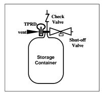
Figure A.3. Typical Compressed Hydrogen Storage System
