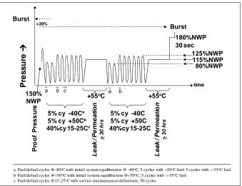
Figure B.5.1.3 Verification Test for Expected On-Road Performance (pneumatic/hydraulic)
