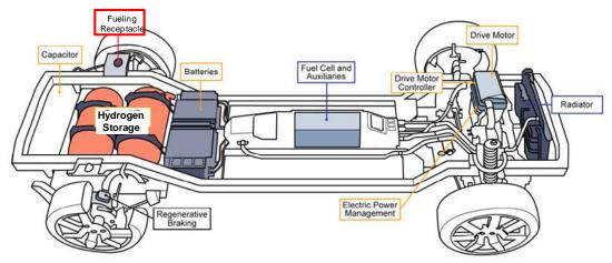
Figure A.2. Example of a Fuel Cell Vehicle
