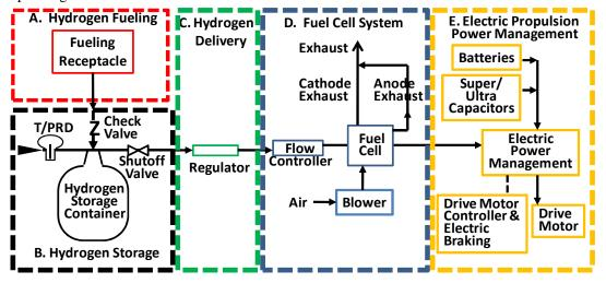
Figure A.1. Example of High-level Schematic of Key Systems in FCVs
