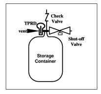
Figure B.5.1.1 Typical Compressed Hydrogen Storage System
