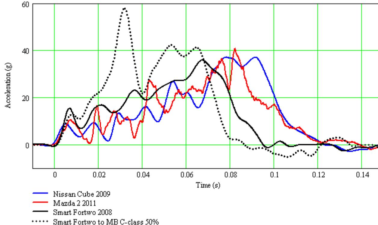
Comment: In the impact to the relatively soft offset deformable barrier (ODB), a considerable amount of the impact energy is absorbed by the ODB. The acceleration levels reaches approx. 35g (solid curves). In the vehicle to vehicle crash, the smaller vehicle experiences considerably higher acceleration levels than in the ODB test (dotted curve).
