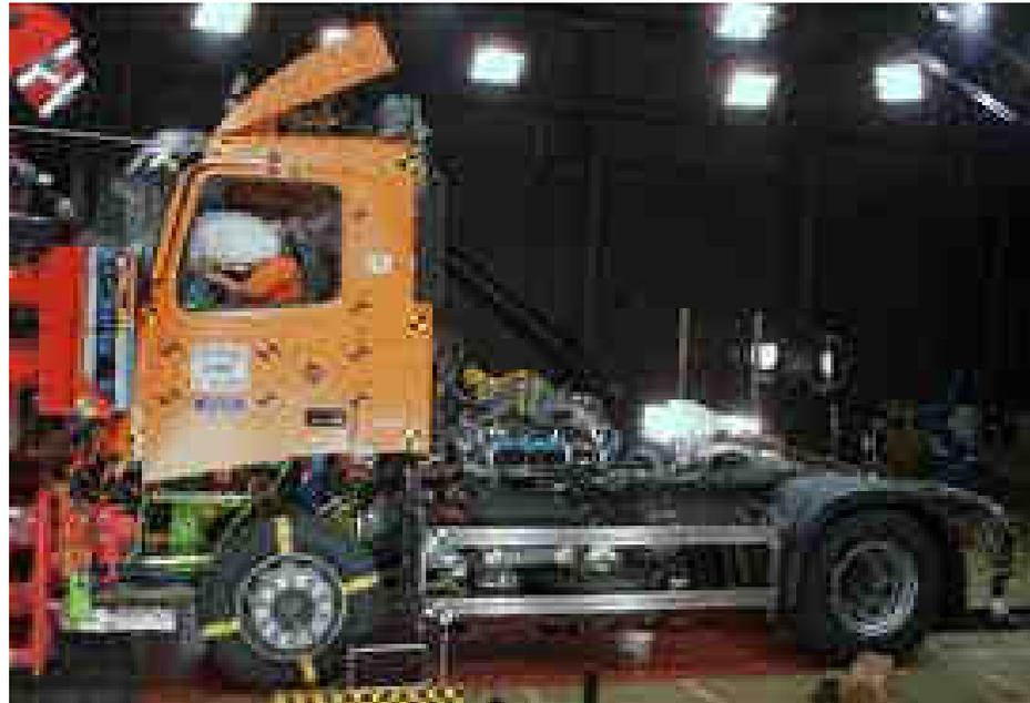
Stiff crash pulses in chassis in collisions to objects and other heavy vehicles, due to short deformation zones.
