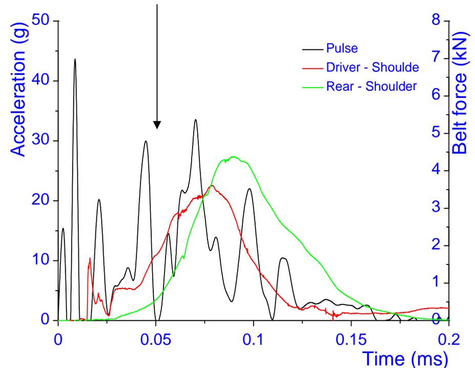
Comment: The smaller vehicle experiences high acceleration levels, even though the counterpart is soft in comparison to the small car. The small vehicle would experience even higher acceleration levels if the counterpart would be of more modern design (often higher stiffness).
