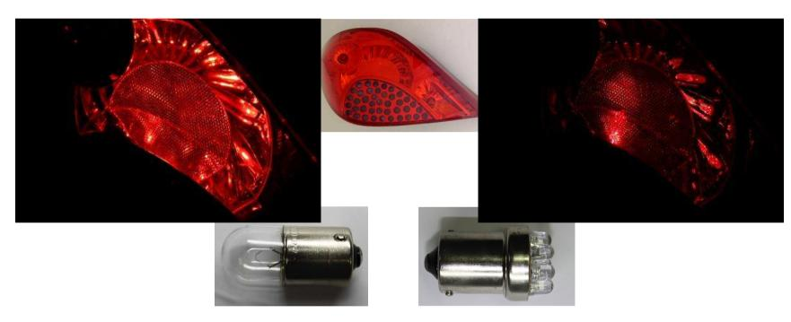
> Luminous output: ok vs. not sufficient
