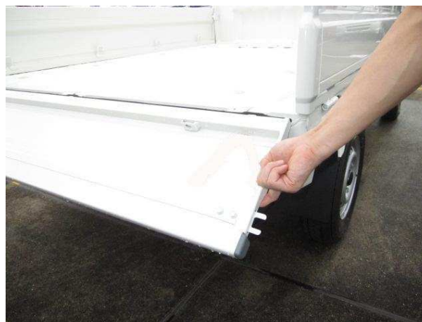
Fig.3 The tailgate is not locked and can easily move.
