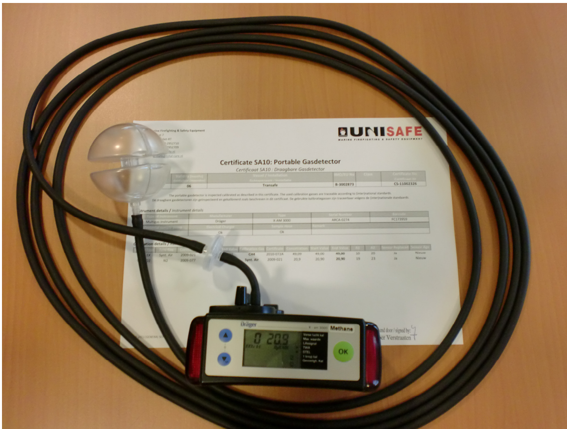
Photo of a combined oxygen/explosion meter with Certificate.
