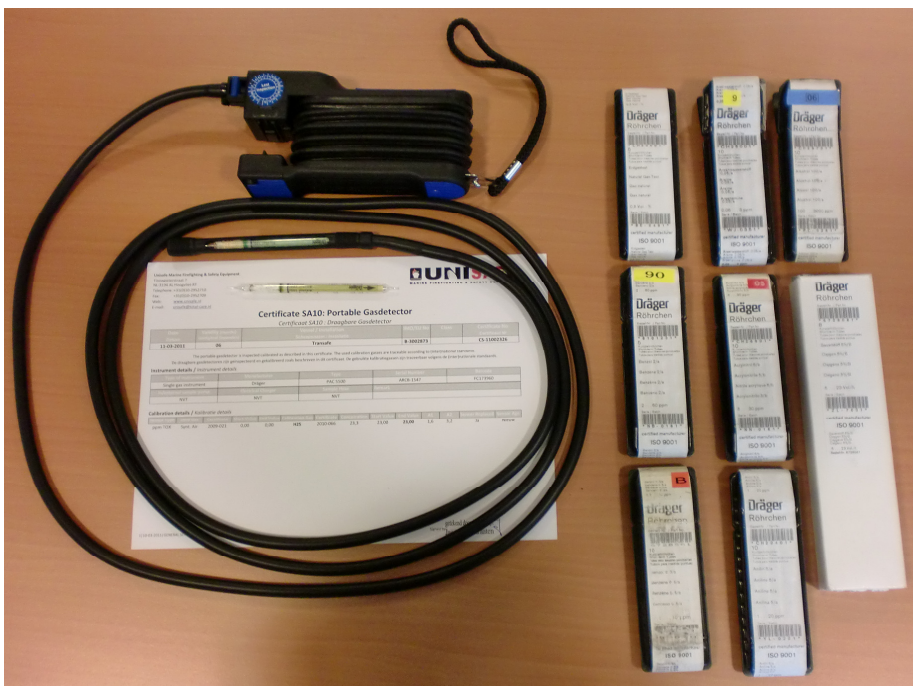
Photo of a toxic gas meter (hand pump) with a number of boxes containing various test tubes and certificate.
