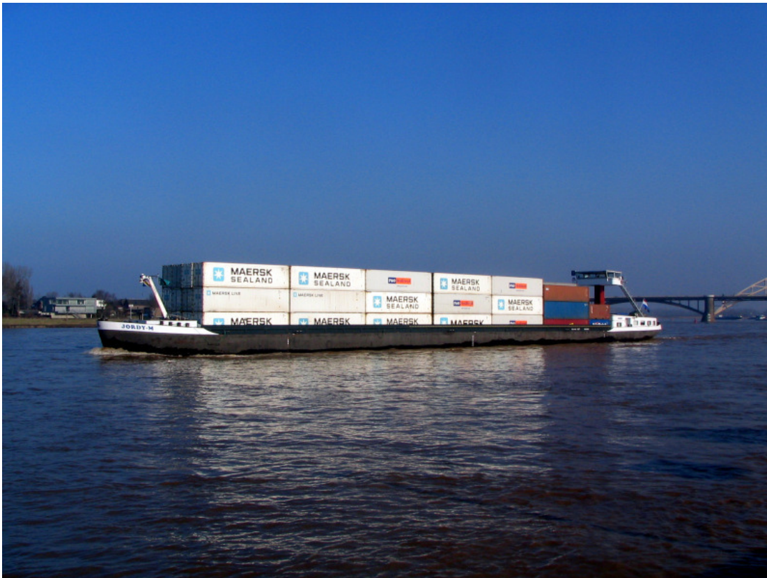
A "standard" container ship "Jordy-M" with the dimensions 110m long x 11.45m wide, 208 TEUs (4 layers).
