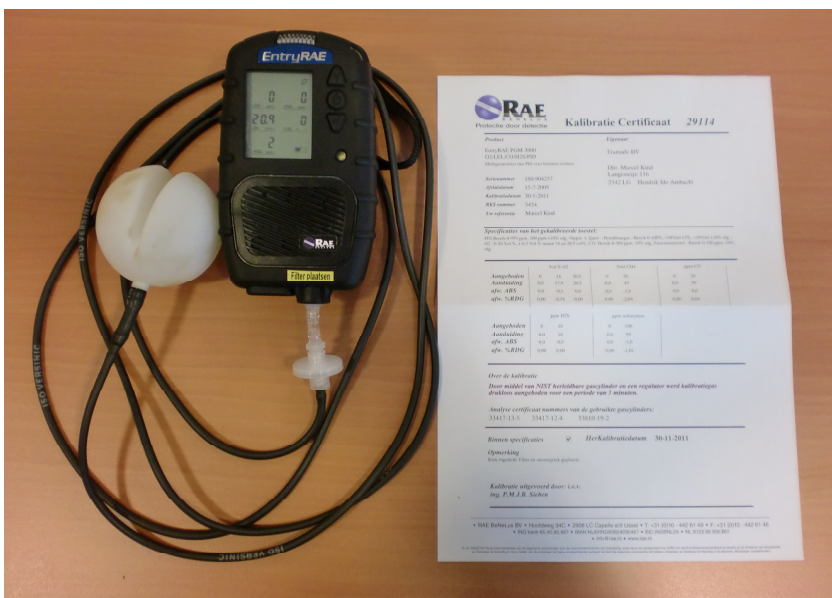
Photo of an example of a PID meter and certificate, which also measures oxygen, explosion, H2S and CO.
