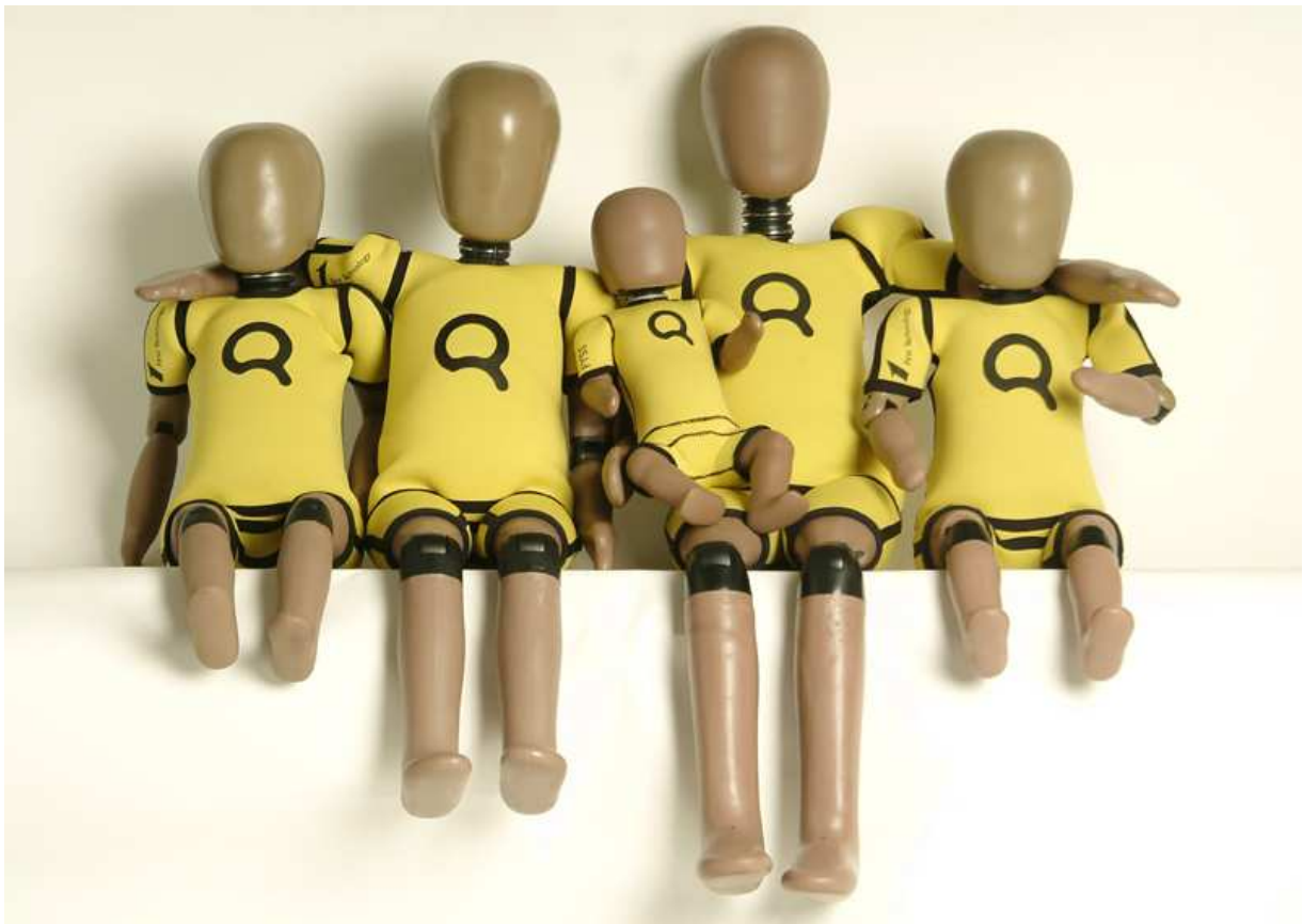
Q-dummy family from left to right: Q1.5, Q3, Q0, Q6 and Q1 [Q10 dummy, being under development, not yet shown]
