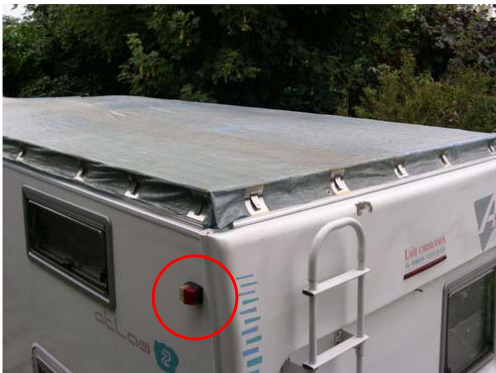
It is clear that in this case the 45° angle of visibility to the inside (imposed by ECE R7 approval as position lamp) is useless.
