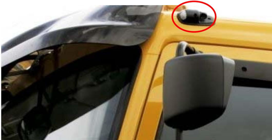
As for the preceding example, it is clear that in this case the 45° angle of visibility to the inside (imposed by ECE R7 approval as position lamp) is useless.
