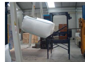
Germany is concerned that the proposed test provisions were designed for IBCs and do not readily correlate to FBCs. For example, Germany believes that it is impractical for FBCs to be tested with the proposed total test weight (6 times its gross mass--> e.g.  $6 \times 14 \text{ to} = 78 \text{ to}$ ). Germany believes the test protocol needs to be modified to be feasible for FBCs.
