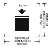
14. There may also be a need for explanatory text to indicate that the mark should be square irrespective of any dimension chosen in excess of the minimum.
