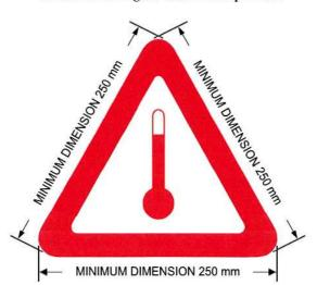
Figure 5.3.4 Mark for carriage at elevated temperature
