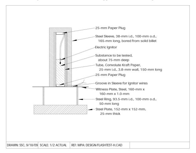
Figure 1 – Modified DDT Test Apparatus for flash compositions
