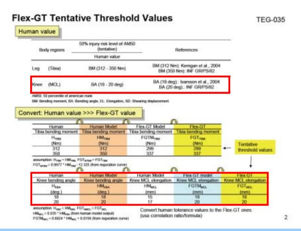
Based on the paper by Iversson et al. (2004) employed by IHRA, and the ESV paper by Konosu et al. (2001), the threshold values for MCL failure were set at 18 and 20 mm.
