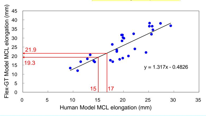
Flex-GT MCL elongation thresholds will be 19-22 mm when the correlation obtained using the FE simulation results with simplified vehicle models INCLUDING those representing high-bumper vehicles is used
