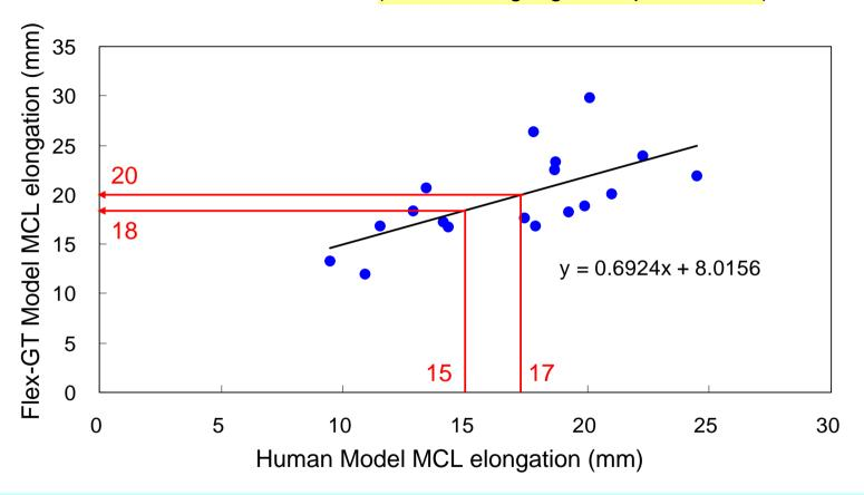
Flex-GT MCL elongation thresholds (18-20 mm) were deduced from the correlation obtained using the FE simulation results with simplified vehicle models **not including those representing high-bumper vehicles**
