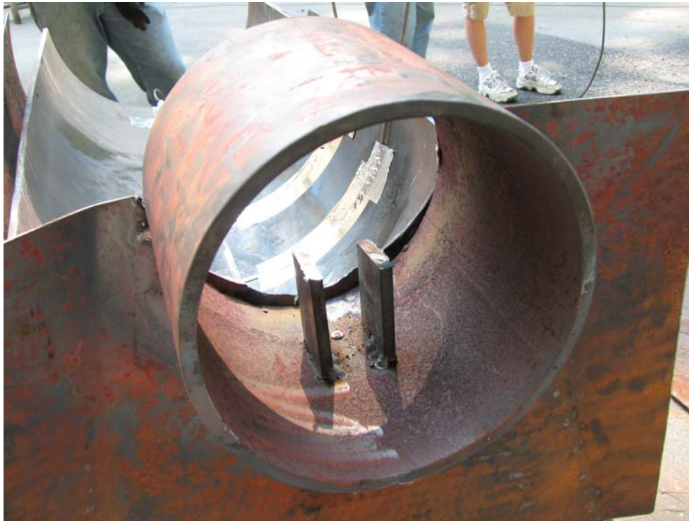
Figure 3 – Temperature transfer “prongs” for the valve end
