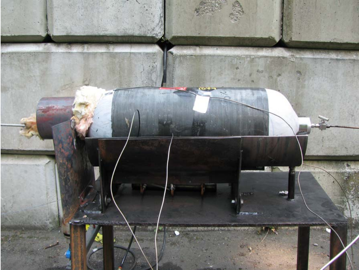
Figure 6 – Fire test of the Dynetek hydrogen tank.
