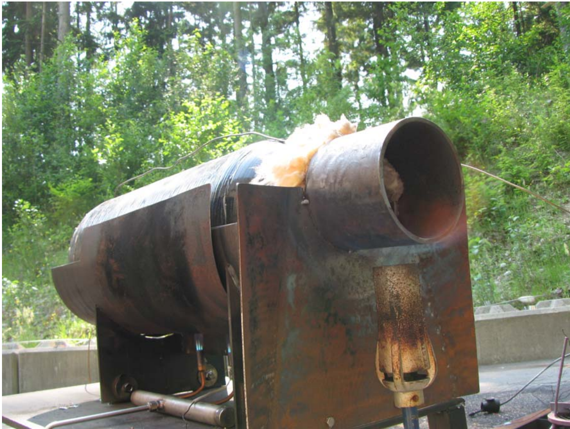
Figure 5 – Test of Type II tank using oxy-propane burners on sidewall and propane torch on valve end.
