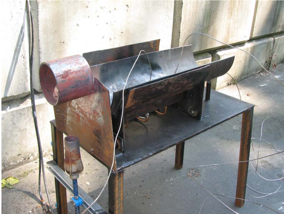
Figure 2 – Overall view of localized fire test apparatus
