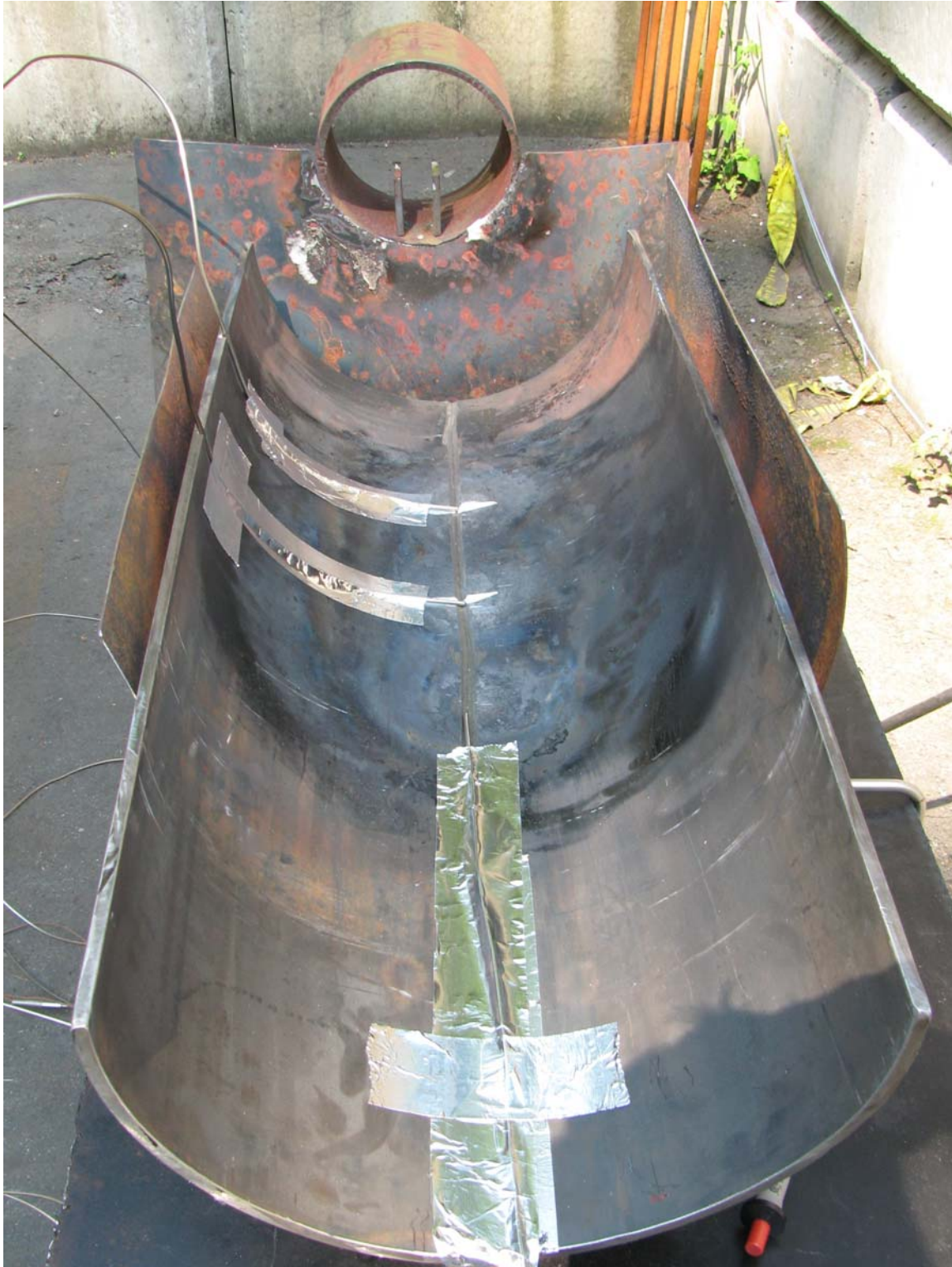
Figure 4 – Thermocouple locations in the metal plate.
