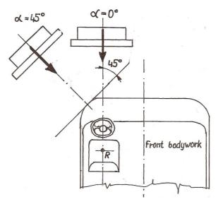
Figure 1. Positions of the impact plate
