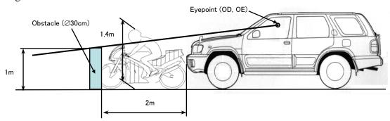
Figure 1. Basis for the Requirement Concerning the Field of Vision under the Japan's Provisions
