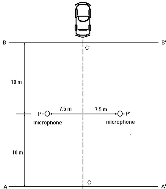
Figure 1. Microphone positions for the measurement
