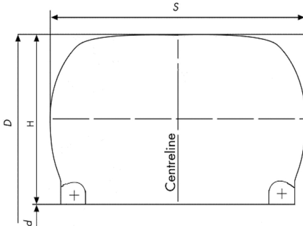
4.4.5.4 Figure 2: Drawing of tyre with rim protector showing rim diameter ( $d$ ), outside diameter ( $D$ ), sidewall height ( $H$ ) and section width ( $S$ ).
