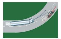
6.5.7.1. The subject vehicle shall approach and pass the target vehicle at a closing speed of 10 km/h when both vehicles are travelling in the centre of adjacent lanes, each 3.5m wide, with the inner marking of the inside lane having a 125m radius of curvature. The target vehicle shall travel at a constant speed of 40 km/h.
