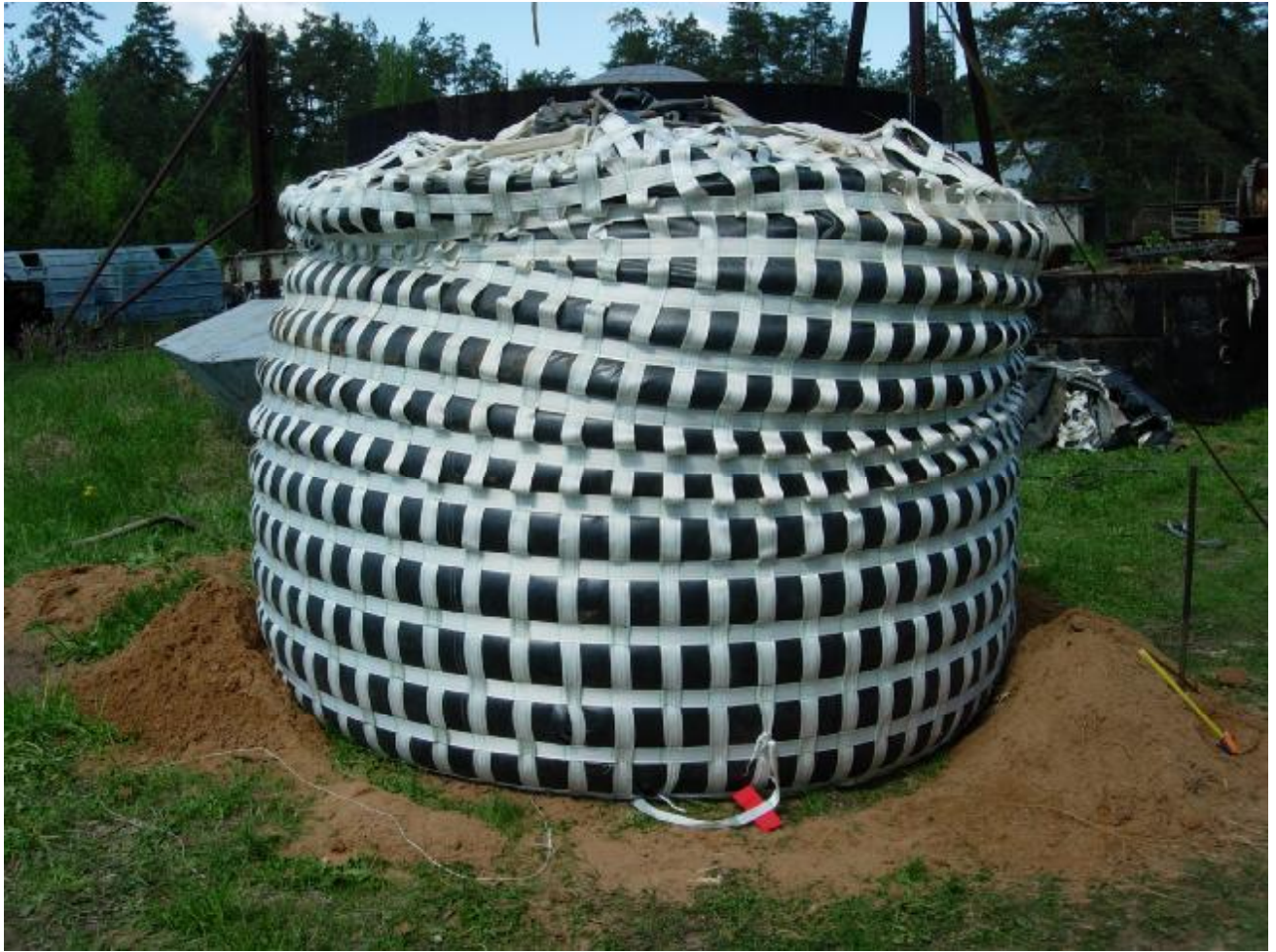
Photo 8.3. Free-fall impact test. The container after the test
