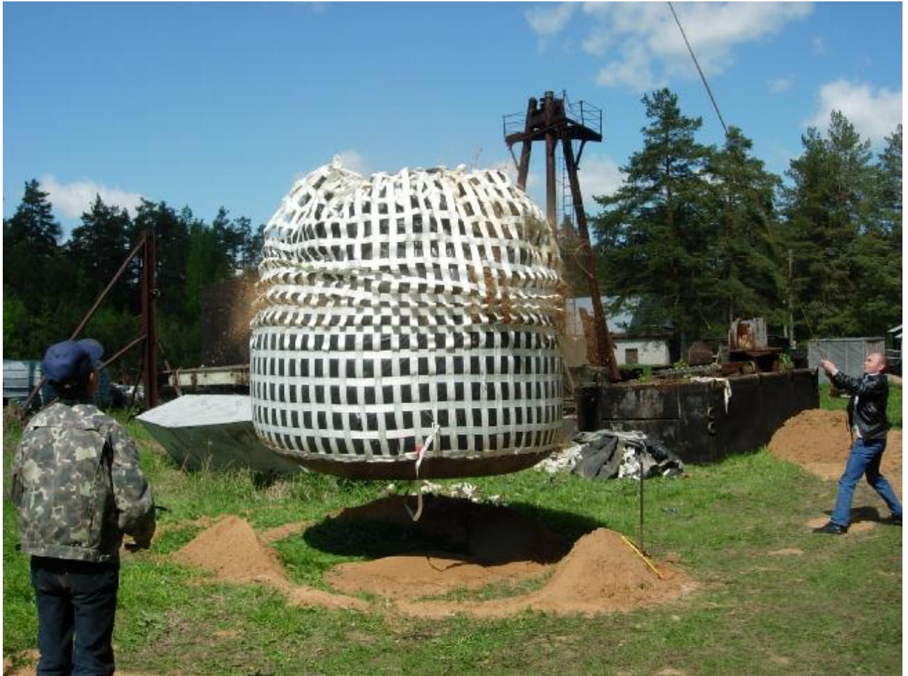
Photo 8.2. Free-fall impact test. Container dropping from the height of 0.8 m
