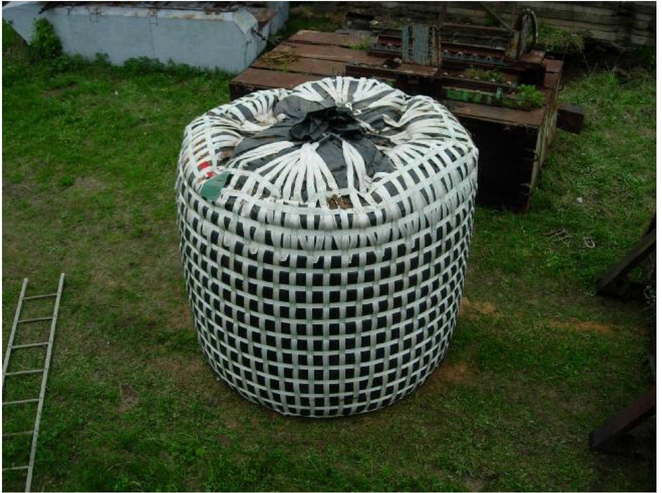
Photo 5.2. Stacking test. Container MK-14-10 after the stacking test
