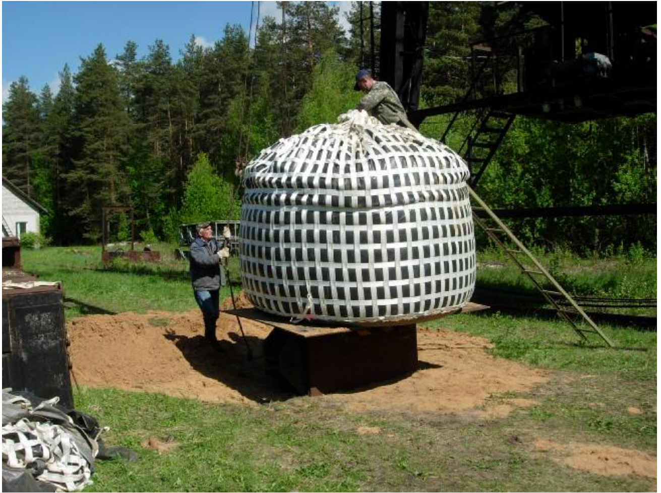
Photo 7.2. Tipping test. The container on the platform at the height of 0.8 m from the floor
