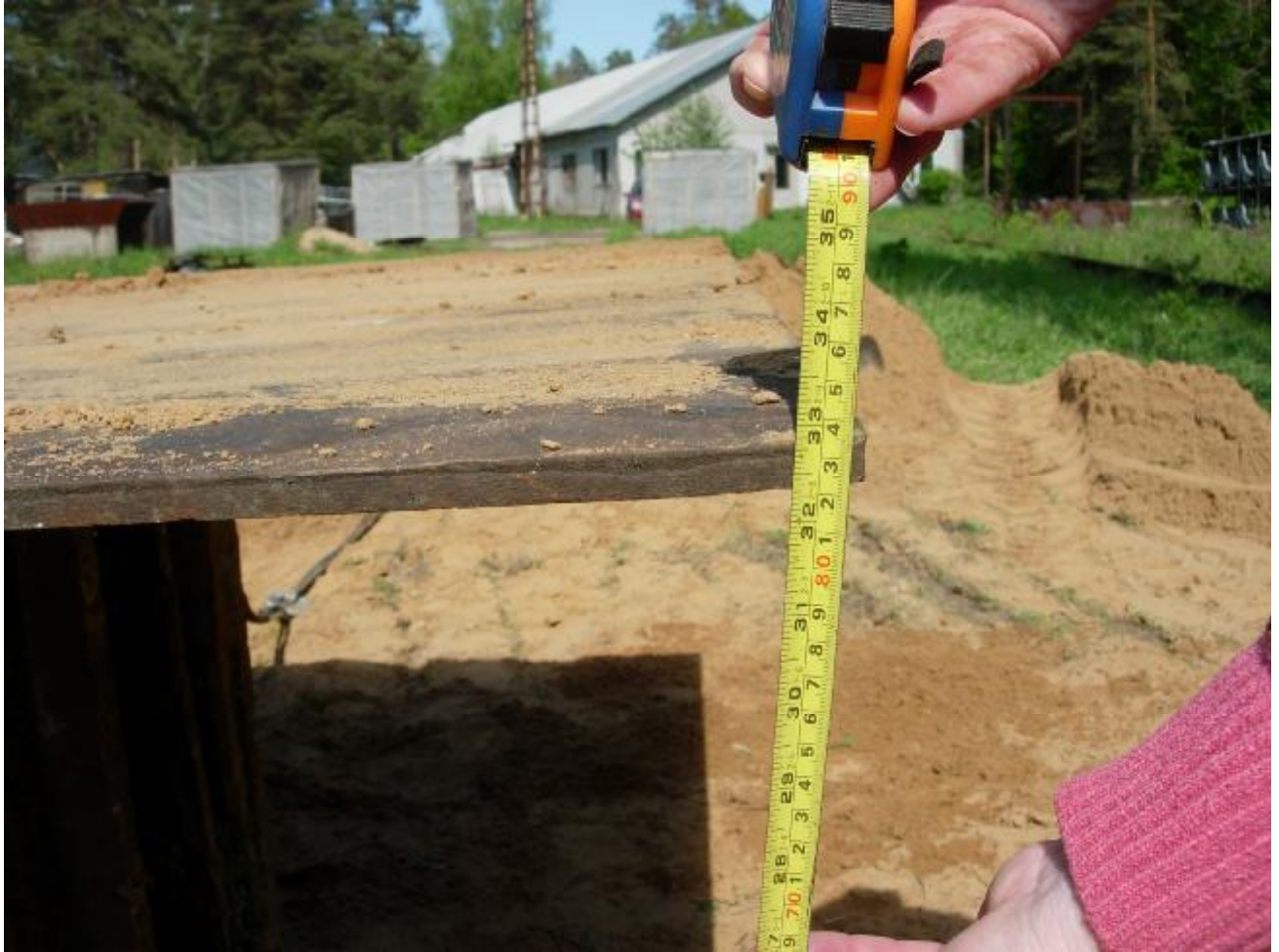
Photo 7.1. Tipping test. Height of the platform for container tipping test is 0.8 m
