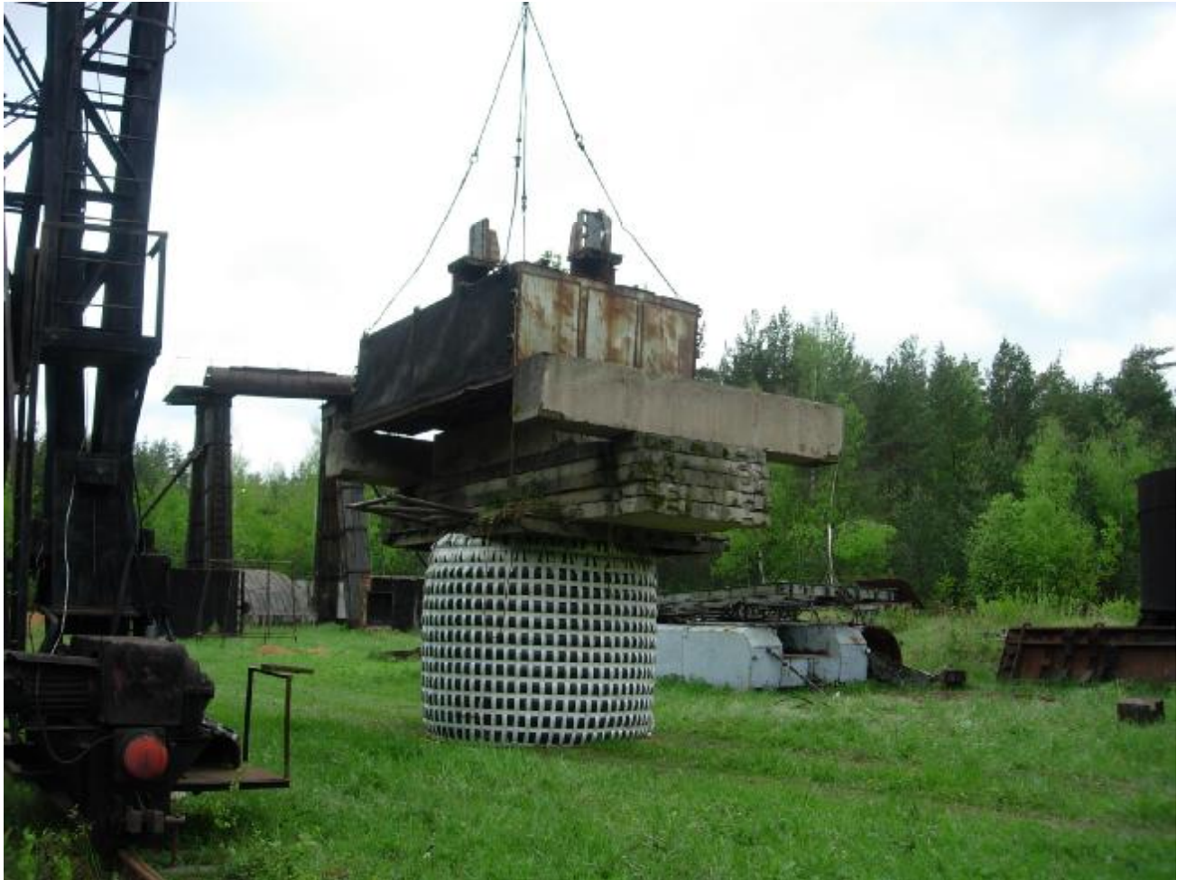
Photo 5.1. Stacking test. Container MK-14-10 under the load of 56 tonnes
