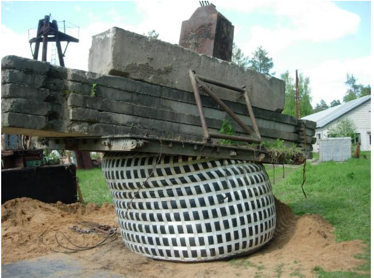
Photo 6.2. Break test. Container dwelling under the load of 28 tonnes
