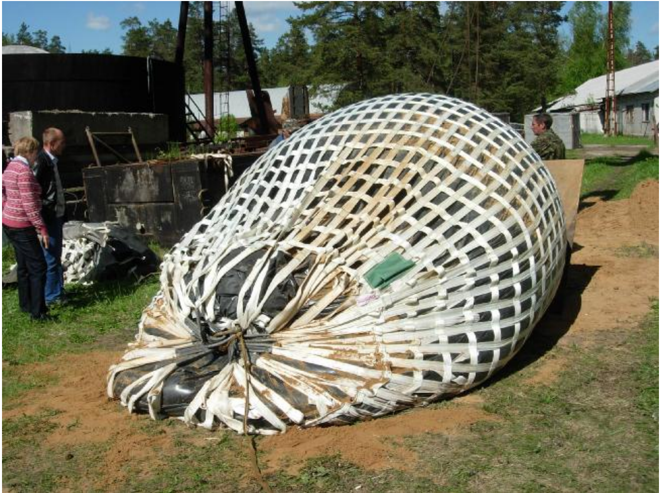
Фото 7.4. Tipping test. The container after the test
