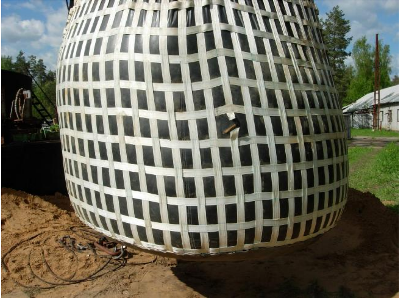
Photo 6.3. Break test. Container dwelling in suspended state
