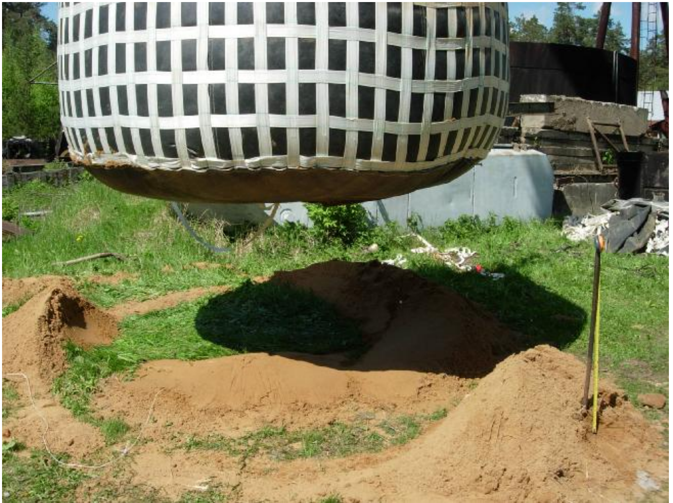
Photo 8.1. Free-fall impact test. The container was lifted to the height of 0.8 m from the floor
