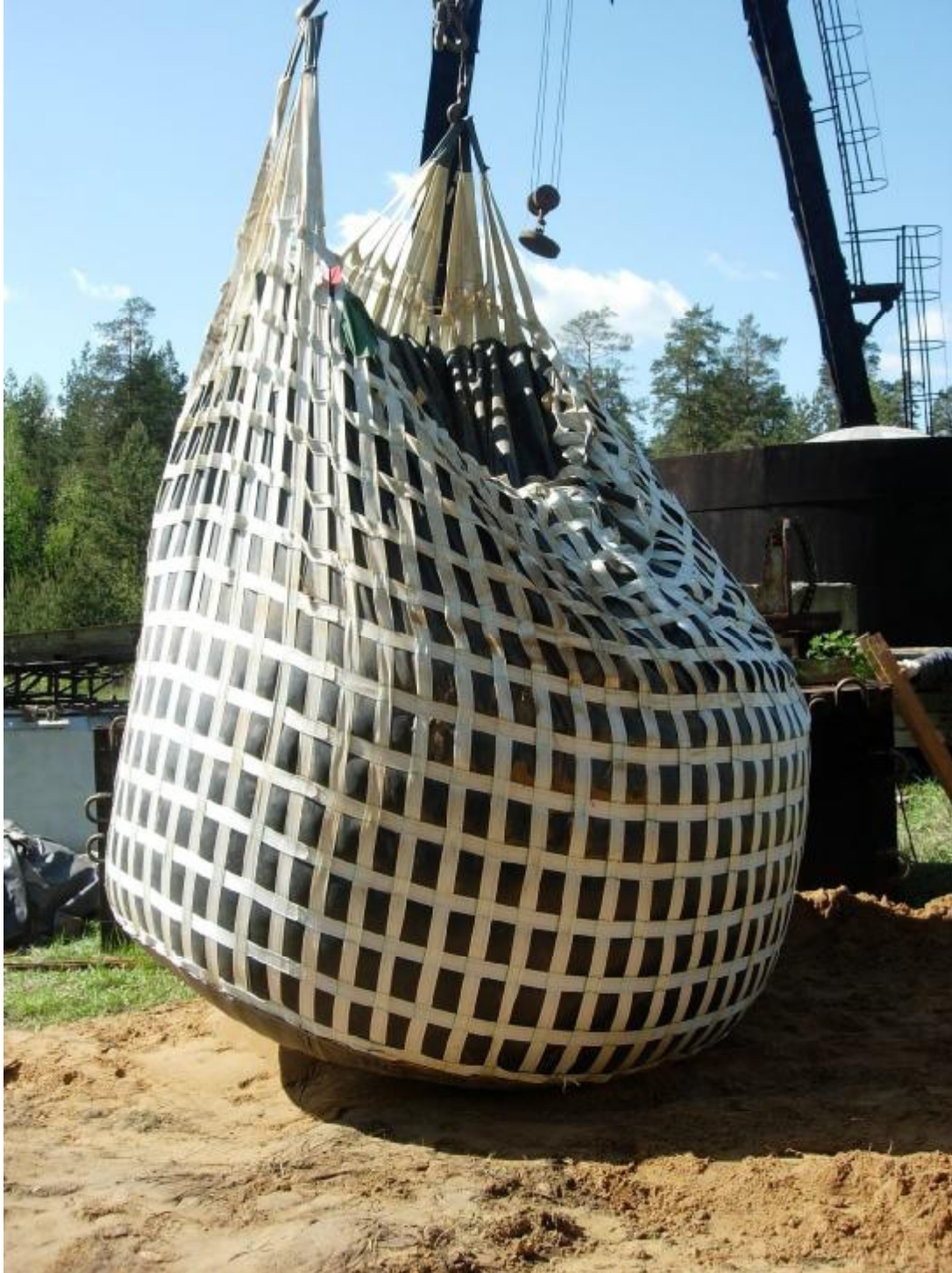
Photo 9.2. Inclination with lifting to vertical position test. The container has been lifted from inclined position by two load-lifting slings with separation from the floor
