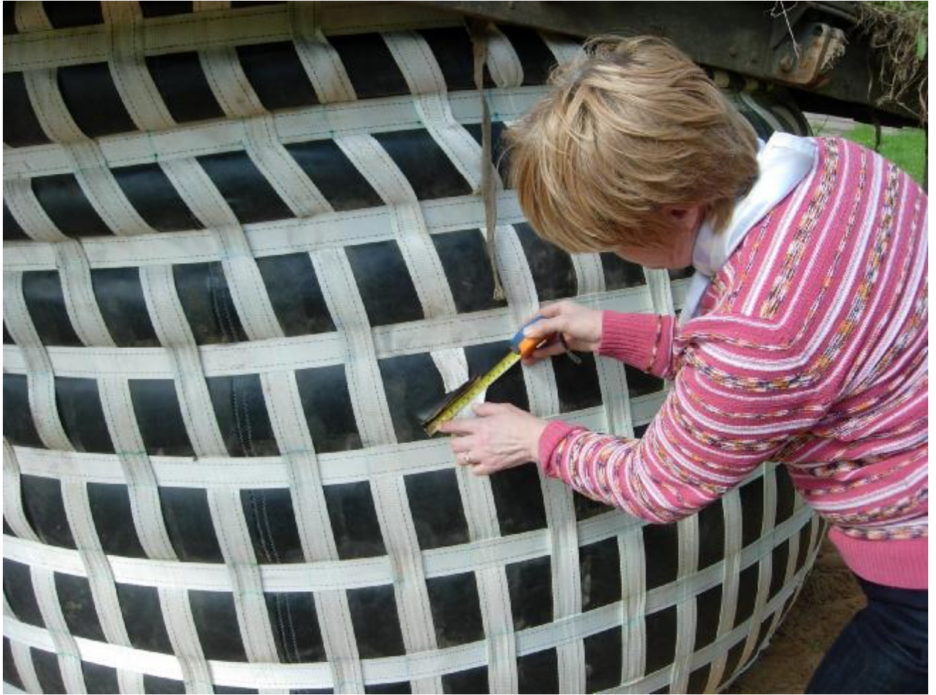
Photo 6.4. Break test. Cut length after the test is 120 mm, without changes
