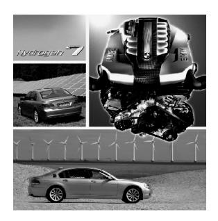
The V12 engine of world's first hydrogen-powered luxury saloon car, which was created in a series development process, represents a further landmark along the road to the hydrogen age. Thanks to sequential hydrogen injection, combined with Valvetronic and a complex operating strategy, the 6.0 I engine develops 390 Nm of torque and a power output of 260 bhp. At the same time it clearly undercuts the toughest emissions regulation worldwide.
