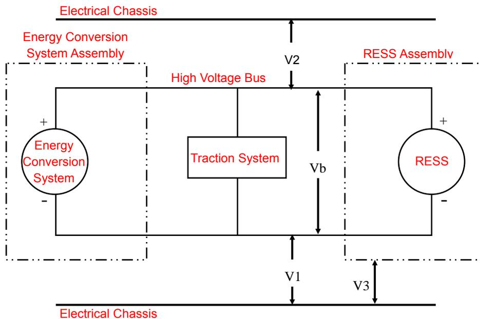
Figure 12: Measurement of  $V_b$ ,  $V_1$ ,  $V_2$
