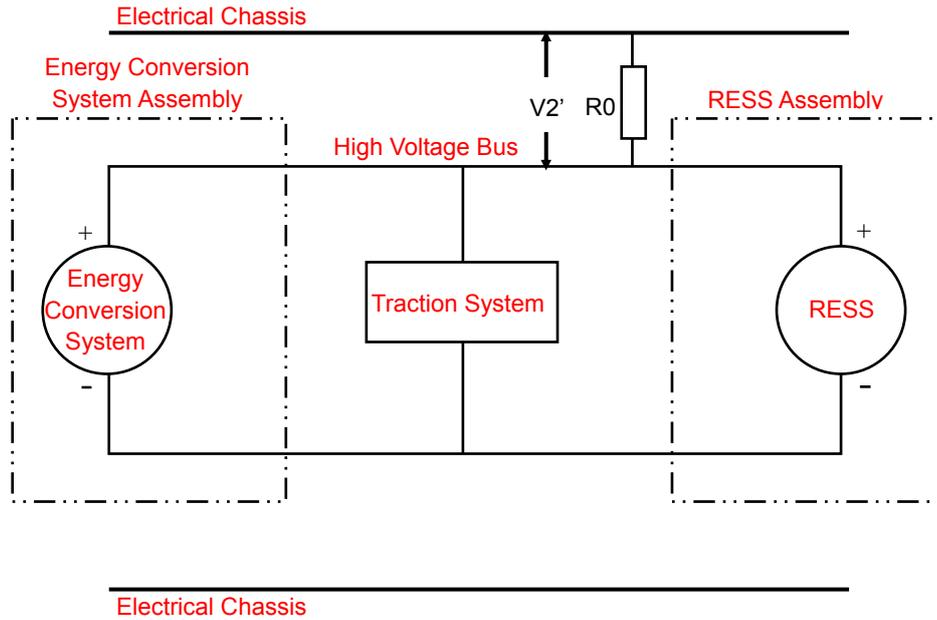
Figure 34: Measurement of  $V2'$
