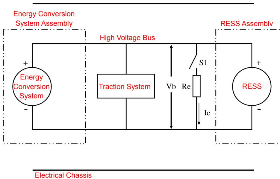
Figure 45: Measurement of high voltage bus energy
