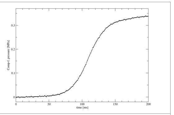
**comp-f:** Analysis of rise-time  $t_{UN2c}$  is not possible since pressures were not achieved. More substance may be required in the test volume.
