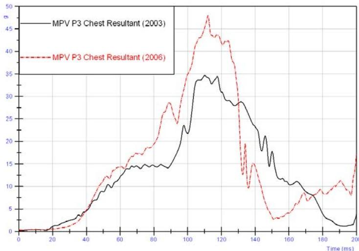
**Figure 7 - P3 child dummy chest resultant acceleration time history, in MPV 2003 and 2006 EuroNCAP tests (same CRS).**
