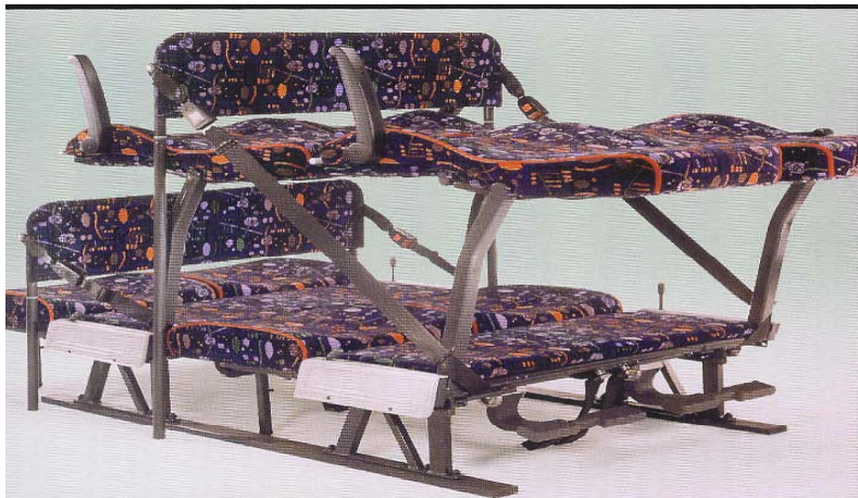
Fig.1. Example of normal seats that can be converted into berths altogether an example of safety partitions attached to the safety belt anchorages of the bus seats.
