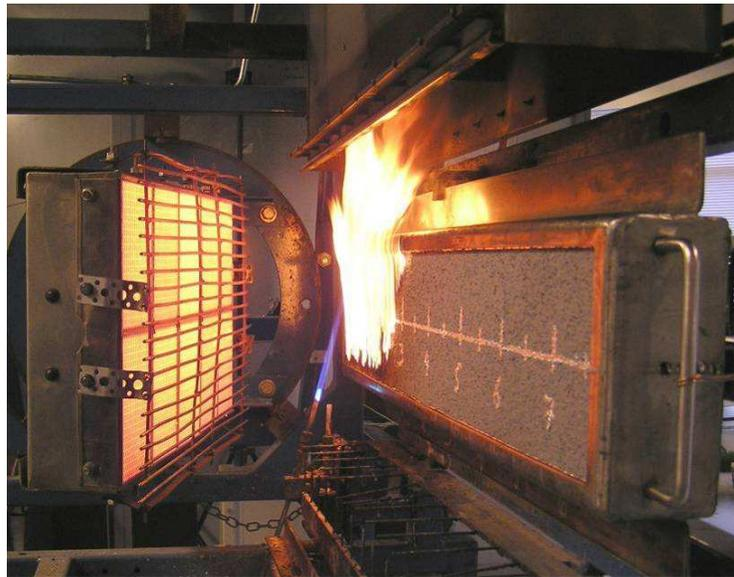
Figure: Photograph of the ISO 5658-2 panel test.
