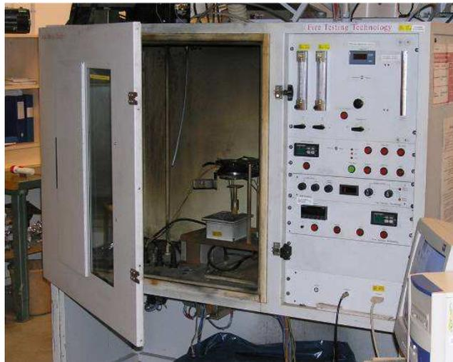
Figure: Photograph of the ISO 5659-2 smoke generation test.
