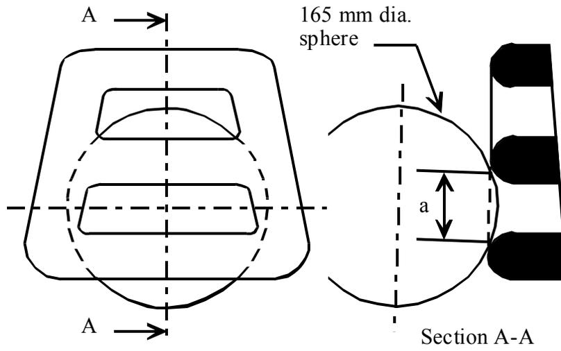
Figure 3 - Measurement of a horizontal gap "a".
