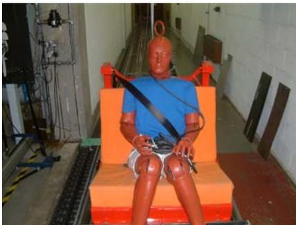
Installation of the Hybrid II dummy on the sled test bench as defined in Regulation No. 44.
