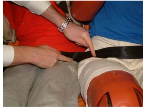
Comparison of pelvic position of P10 and 50th percentile adult male dummies. Recorded pelvis vertical measurement was 34 mm lower for the P10.
