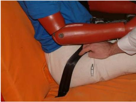
Vertical Pelvic position at load bearing point of Hybrid 2 - 50th from Cr axes. Recorded distance is (191 mm)
