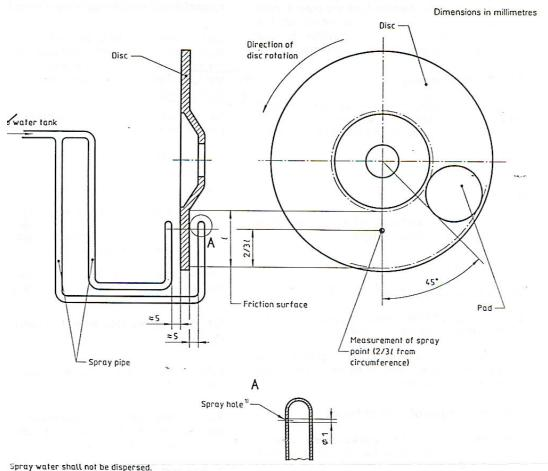
The disc brake water spray equipment shall be installed as follows:
