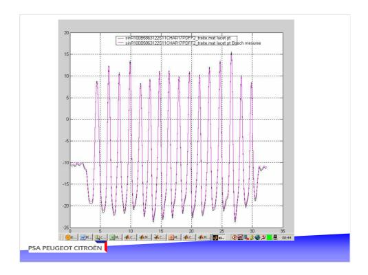
In black we have the measurement obtained with a yaw rate sensor that complies with ISO requirement.
