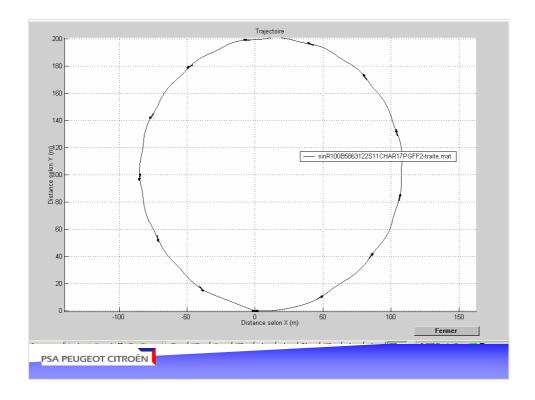
The trajectory is a circle of 100 meter radius + a slalom of 3 meter amplitude.
