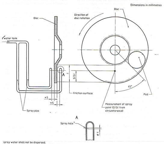
(d) Each brake is fitted with water spray equipment(i) Disc brakes: Sketch of water spray equipment:
