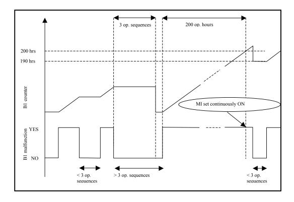
Figure C2: Illustration of the B1 counter activation principles
