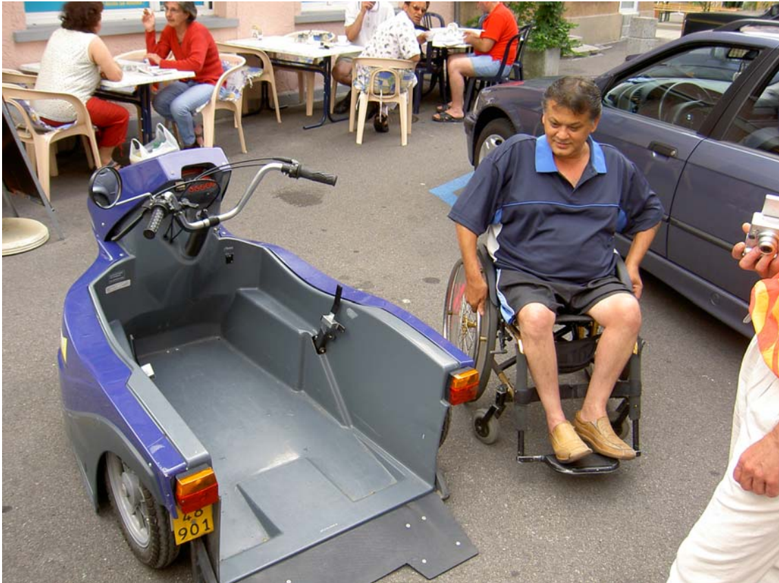
Moped designed to contain a wheelchair. This type of vehicle may be admitted on surfaces designed for walking.
