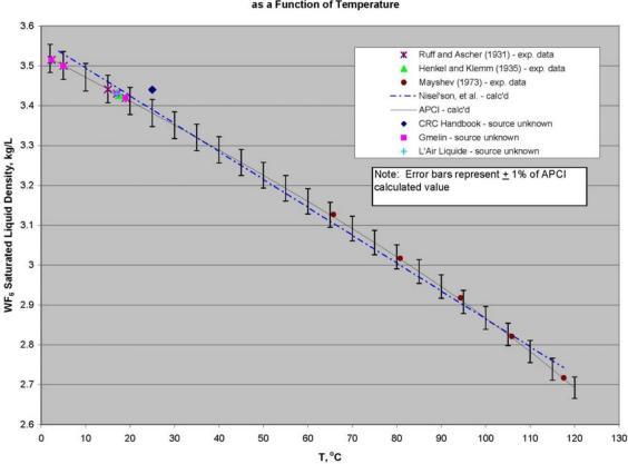
Comparison of WF<sub>6</sub> Saturated Liquid Density Experimental Data and Predicted Values as a Function of Temperature
